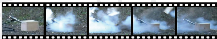
The sequence above demonstrates ABL3000 being fired from the optional lightweight stand against a simulated target. Note, no movement!
